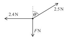
A particle rests on a smooth horizontal surface. Three horizontal forces of magnitudes 2.5 N, F N and 2.4 N act on the particle on bearings  $\theta^{\circ}$ , 180° and 270° respectively (see diagram). The particle is in equilibrium.
