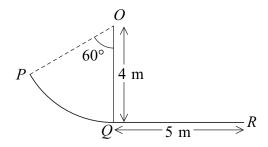
Simon, a child of mass  $32\,\mathrm{kg}$ , uses the slide, starting from rest at P. The curved section of the slide, PQ, is one sixth of a circle of radius 4 metres so that the child is travelling horizontally at point Q. The centre of this circle is at point Q, which is vertically above point Q. The section QR is horizontal and of length 5 metres.
