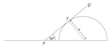
The rod is on the point of slipping when it is inclined at an angle of  $30^{\circ}$  to the horizontal.
